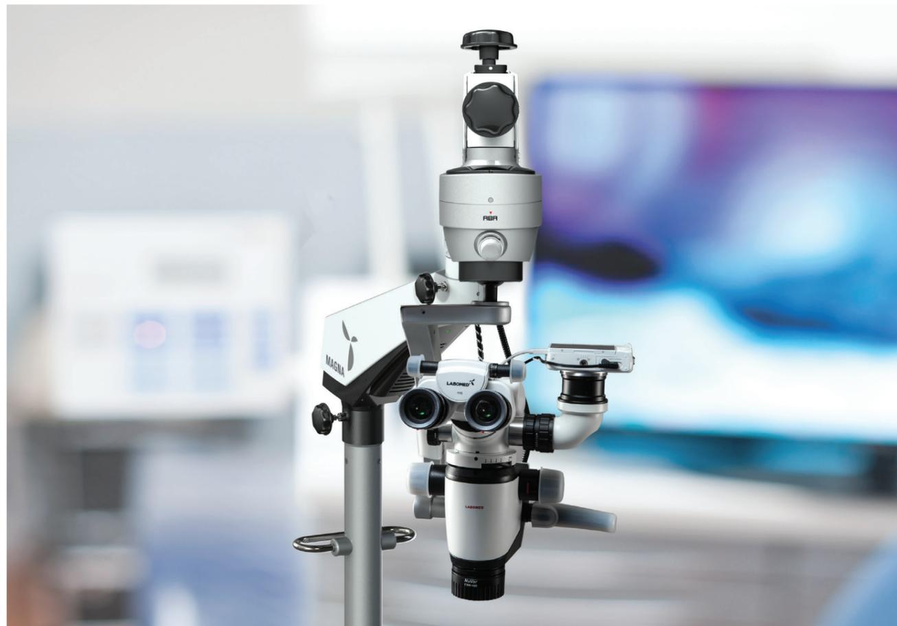
Both the ergonomic handle and carrier arm are equipped with a brake release button, appealing to both right and left handed users. The *NuVar* variable objective comes equipped with a responsive control collar for smooth adjustments to focal length.
